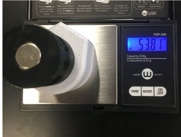
Finding mass of 3D catcher, ball and magnet.
