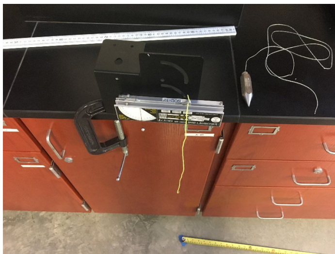
mini-launcher setup showing protractor, spot marked on the floor beneath release point for the ball, plumb bob, meter stick and tape measure. not shown: landing spot with carbon paper.
