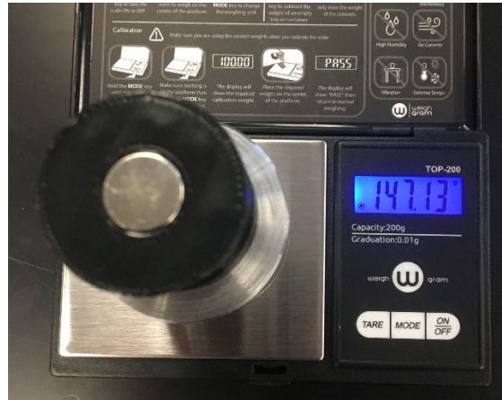
Measuring mass of the catcher, magnet and ball.
