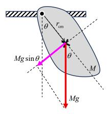
Now we can apply the "rotational equivalent of Newton's  $2^{nd}$  law",  $\tau = I\alpha$ , where  $\tau$  is the torque exerted by gravity and  $\alpha$  is the angular acceleration.
