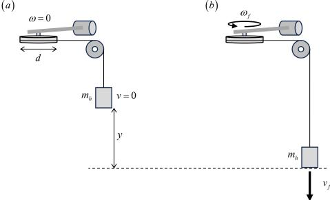
In (a) we show the initial state of the machine, with the hanging mass  $m_h$  suspended a distance y above its final position. Note that the string is wrapped around the hub of diameter d here.
