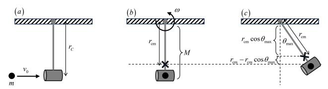
In (a) our projectile of mass m is moving with speed  $v_0$  prior to impact. We also label  $r_C$ , the distance from the rotation axis to the center of the catcher.
