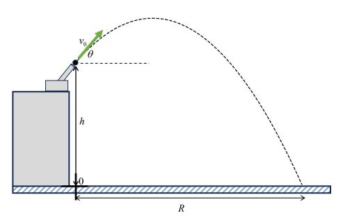
We place the origin directly below the projectile, at ground level. Starting with a horizontal analysis of the motion, we obtain an expression for flight time in terms of R,  $v_0$  and  $\theta$ :
